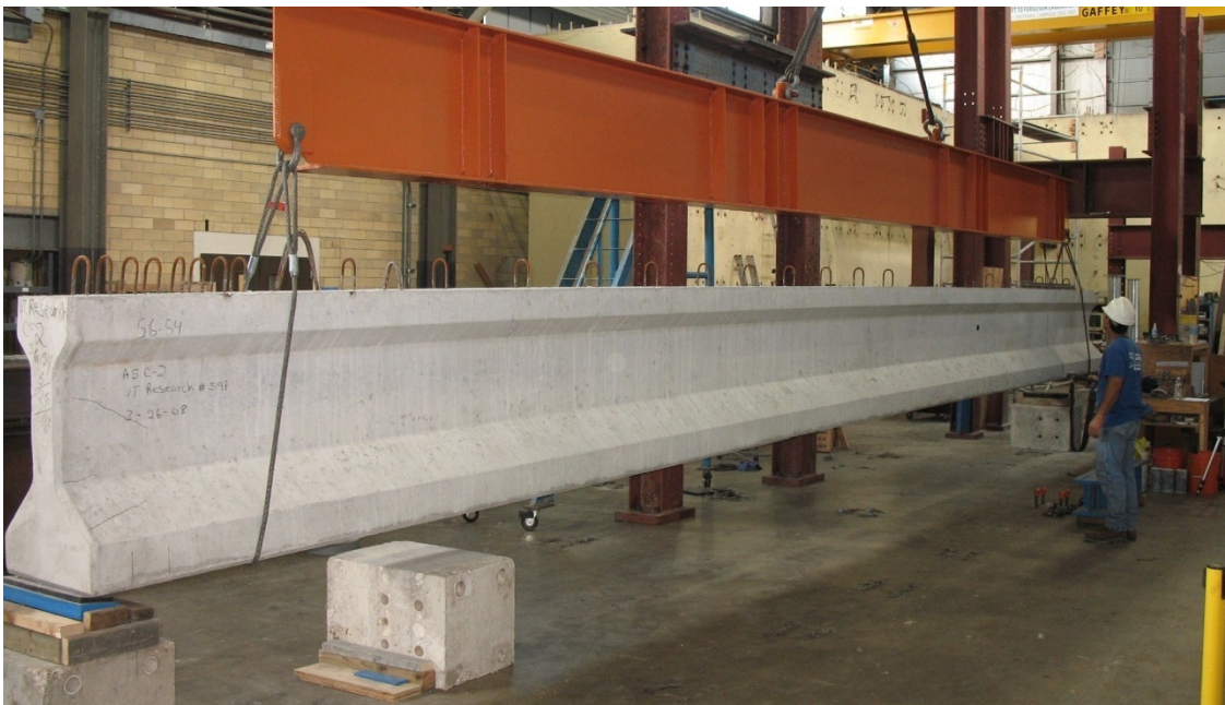
Figure 3.13 Removal of Failed C-Beam Specimen out of Test Setup
