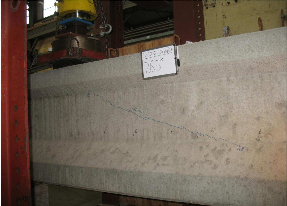
Figure 5.4 First Web-Shear Crack on Beam CD-60-2
