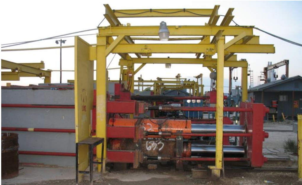
Figure 3.7 Typical Live End of Stressing Bed
