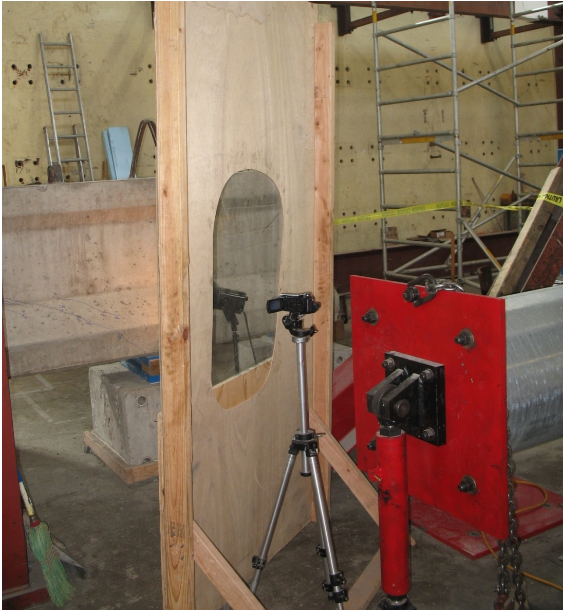
Figure 4.10 Video Camera Setup behind Protective Shield
